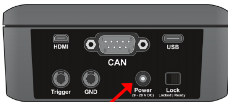
Power socket on the rear of the device
