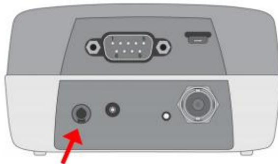
GND socket (4 mm) on the rear of the device
