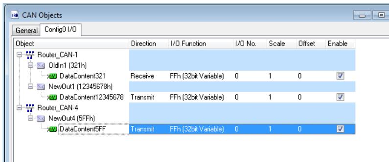
1. I/O-Function: FFh 32 bit variable (used for temporary storage of the content).
