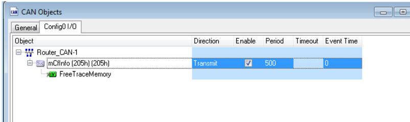
1. Direction: Transmit (the PCAN-Router Pro shall be transmitter).
