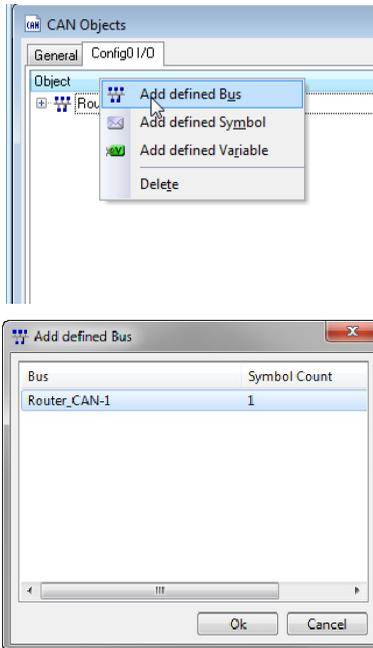
**Reaction:** The previously defined global CAN bus Router\_CAN-1 (along with his contained message mCfInfo and 32 bit variable FreeTraceMemory) will be imported into the configuration Config0.
