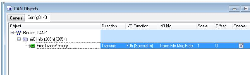
1. I/O-Function: F0-Special In (this is the source: an internal firmware variable).
