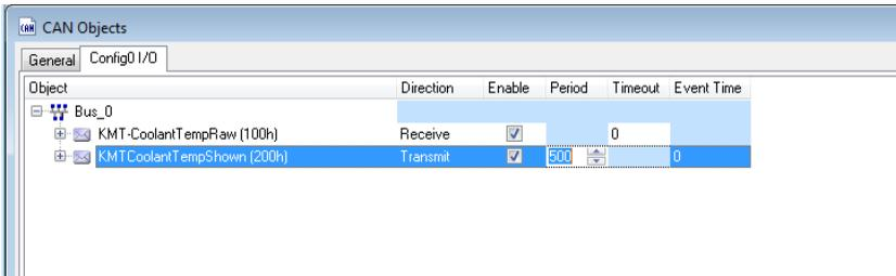
1. Direction: 0x100 is received, 0x200 is transmitted.
