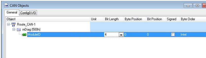
Importing of the message and signal into the configuration (cycle time 500 ms):
