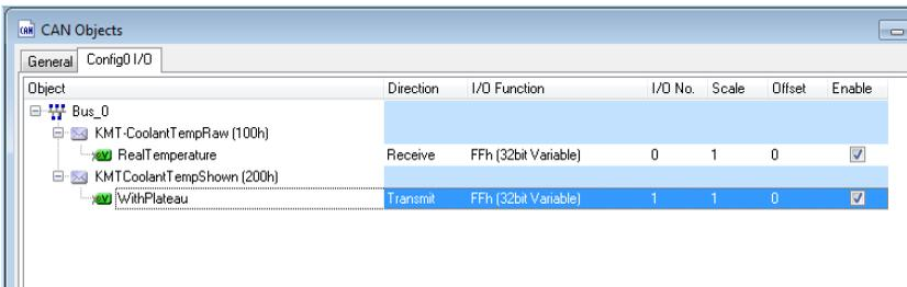
I/O-Function, I/O-Number: The signal RealTemperature from message 0x100 is transferred into variable #0, the modified result WithPlateau is transferred with message 0x200.
