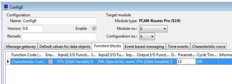
1. Function Code: Characteristic curve (a special function block for this purpose).
