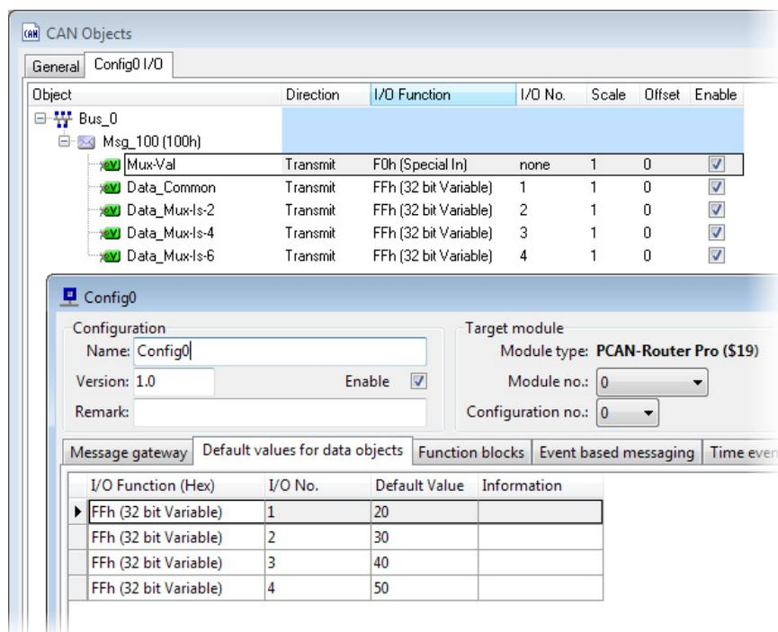
**Remark:** The resource Special In (F0h)/none is assigned to the multiplexer variable Mux-Val. This means that the variable is set to the next Multiplexed variable with each transmission of the CAN message (here every 200 ms). Thus, the Multiplexed variables are transmitted in sequence.
