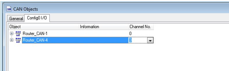
1. Channel-Number: 0 (for Router\_CAN-1) and 3 (for Router\_CAN-4).
