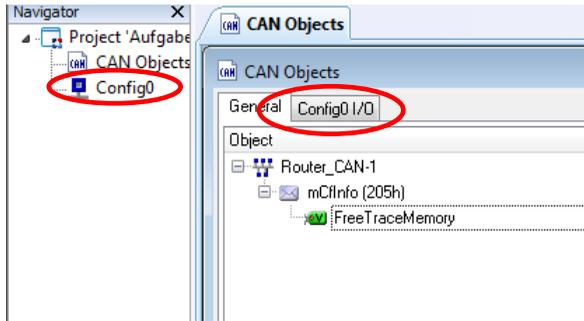
**Activity:** The globally defined CAN message shall be used in this configuration here. Therefore it must be imported. Click on the new tab Config0 I/O (for bringing it into the foreground) and select from the context menu (right click) **Add defined Bus:**
