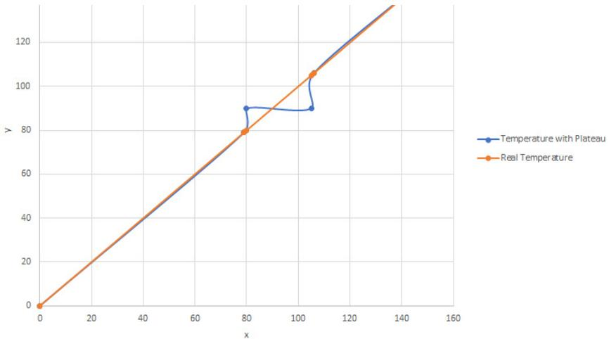
**Information:** For implementing such a behavior, the function block "characteristic curve" is suitable. It recalculates any incoming value by means of a X->Y list (thus creating that plateau).
