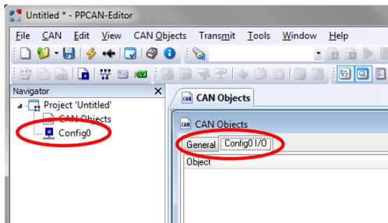
**Activity:** A double-click on this icon will open the configuration window. Here, e.g. default values for data objects can be set, like routing instructions etc. Change to Default values for data objects by selecting that tab. Then a new record must be added here by either selecting menu entry **Edit -> Add record** or selecting **Add record** from the context menu:
