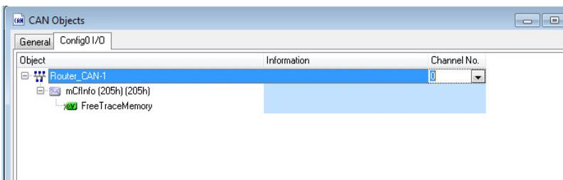
1. Channel-Number: 0 (the hardware CAN channels are numbered 0-3 internally).
