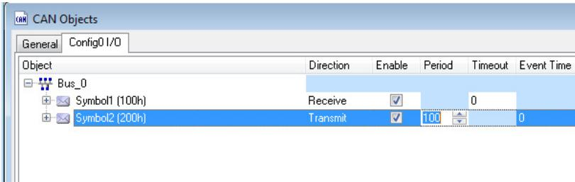
1. Direction: 0x100 is received, 0x200 is transmitted by the PCAN-Router Pro.
