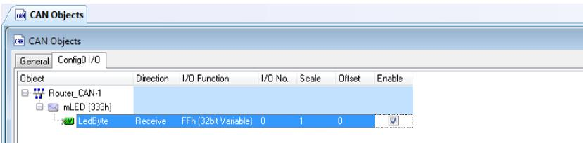
I/O-Function, I/O-Number: The signal LedByte from the message 0x333 is transferred into the variable #0.
