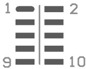
Figure 7: Pin assignment J4 JTAG
