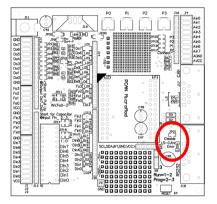
Figure 11: Position of the error status LED for Low-speed CAN, and position JP21
