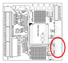
Figure 21: Position of the RS-232 connector
