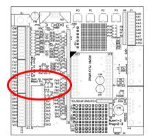
Figure 15: Area of the frequency inputs with the associated DIP switches, LEDs, and the solder positions for adjustments
