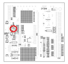
Figure 5: Positions JP23 and JP24 on the bottom side of the Evaluation Board
