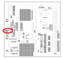
Figure 7: Position JP32 on the bottom side of the Evaluation Board
