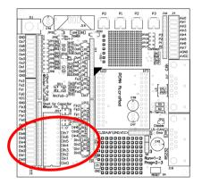
Figure 14: Area of the digital inputs with the associated DIP switches and LEDs
