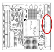
Figure 2: Position of the CAN connector
