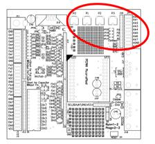
Figure 18: Area of the analog inputs with the associated potentiometers and the solder positions for adjustments
