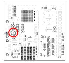
Figure 9: Positions JP28 and JP29 on the bottom side of the Evaluation Board
