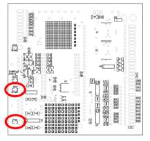
Figure 23: Positions JP26 and JP27 on the bottom side of the Evaluation Board
