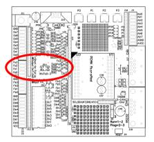
Figure 17: Area of the frequency/PWM outputs with the associated LEDs and the solder positions for adjustments
