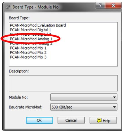
Figure 5: PCAN-MicroMod Configuration: selection of the Analog 1 motherboard
