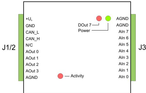
Figure 4: Ports of the Analog 1 motherboard
