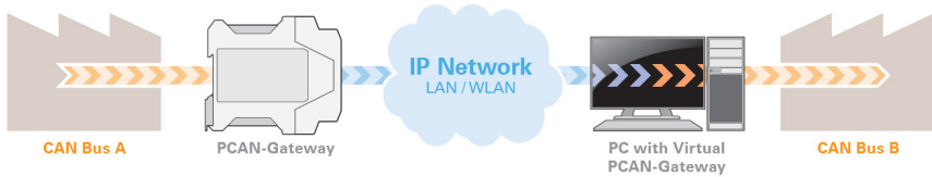
Figure 2: Connection via the Software Virtual PCAN-Gateway
