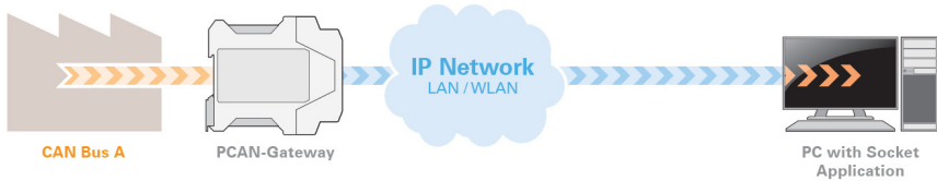
Figure 3: Connection via a Socket Application
